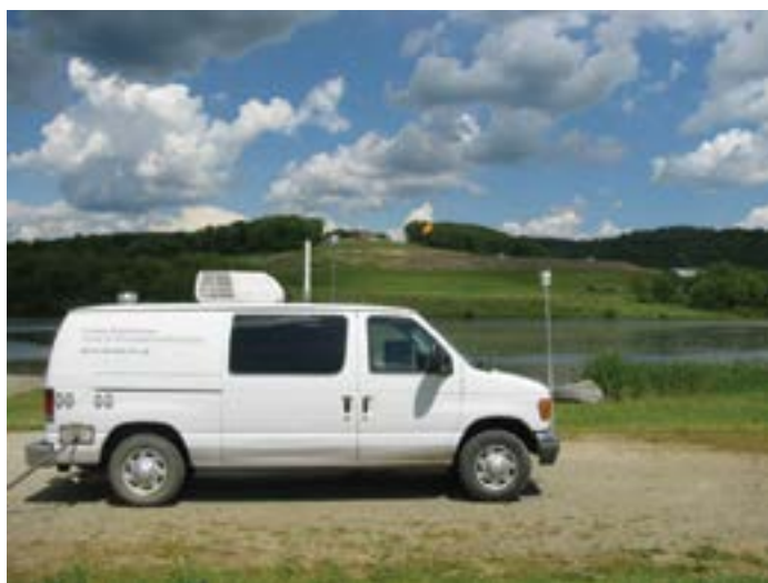
Photograph of the mobile air quality laboratory sampling at a Marcellus Shale site. The tubes exiting the roof of the van are the sample lines, and the instruments are inside. The pole on the front of the van is a weather station that collects temperature and wind speed data. The Marcellus site was a newly drilled well that was flaring at the time of sampling. It is the orange flame in the background.
