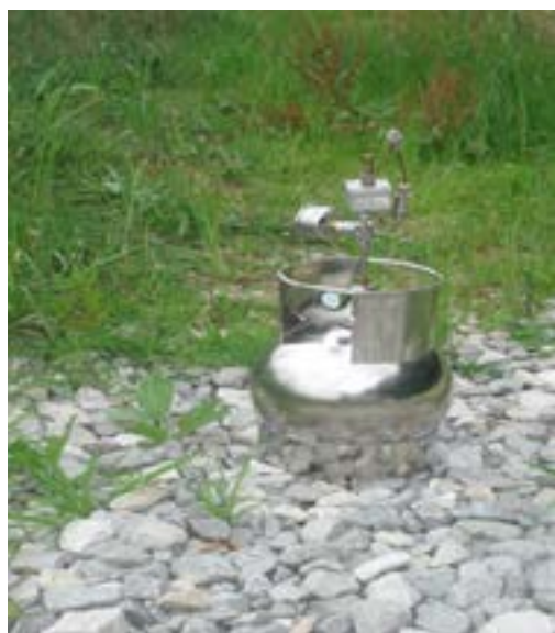
This summa canister samples air near natural gas drilling operations.
